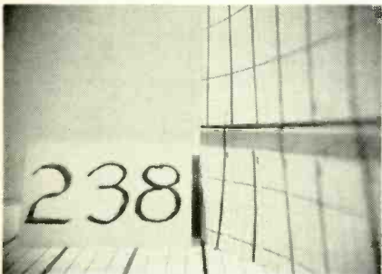
Fig. 7—Test of the camera with a 238-mm supplementary lens. Camera focuses at slightly less than 9 inches and covers a field approximately 4 x 5 in.
