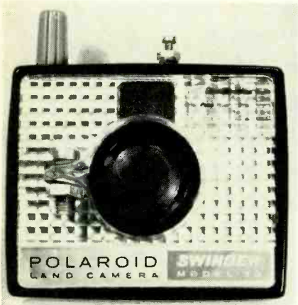
Fig. 6—Front of the modified camera. A plastic cable clamp holds supplementary lens in place. The added stop screw is on the top just to the right of center.
